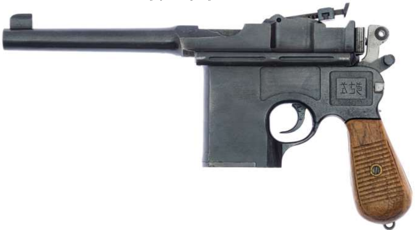
Photos above and below. Right and left sides of .45 caliber Shanxi Type 17 pistol. Note how the magazine extends well below the triggerguard in order to accommodate the larger .45 cartridges. Photos courtesy of Joh. Springers Erben, Vienna, Austria.
