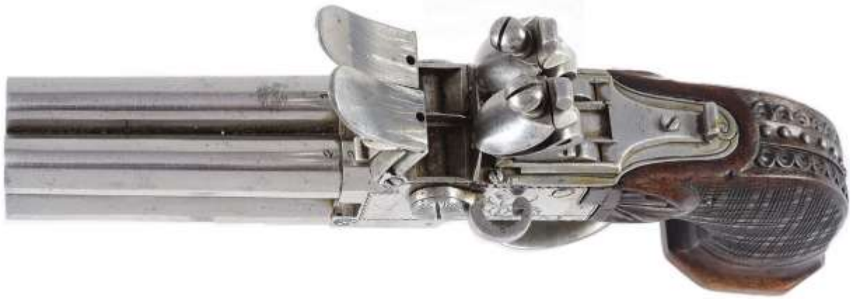
Belgian 4-barrel double flintlock tap action pistol. Note the holes for pins in the two frizzens. Photo courtesy of Morphy Auctions.
