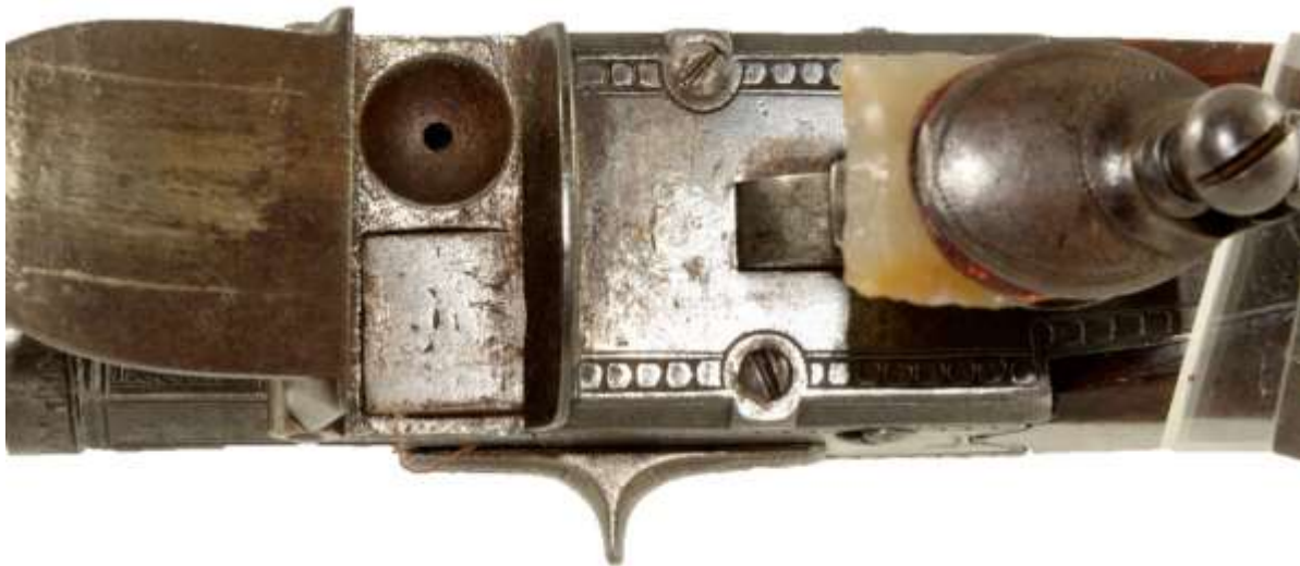
Tap action side by side pistol by John Henshaw of Cambridge. Tap is closed exposing the touchhole to right barrel. Photo – Ivonne Pabon-Marrero.
