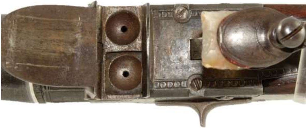
Tap action side by side pistol by John Henshaw of Cambridge. Tap is open exposing touchhole to left or both barrels. Photo – Ivonne Pabon-Marrero.
