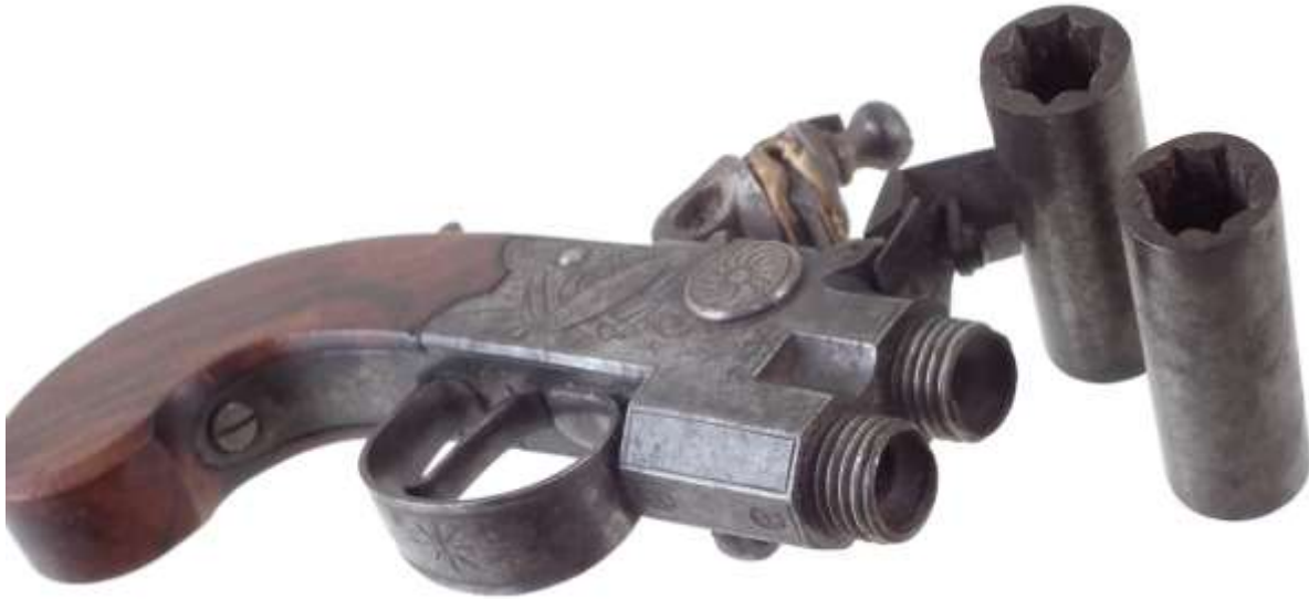
Two barrel, tap action pistol by Henry Nock. 1 3/4" long, 120-bore barrels are turned off. Note the close proximity of the male threaded bushings that form the chambers and that the barrels are screwed on to. Photo - private collection.
