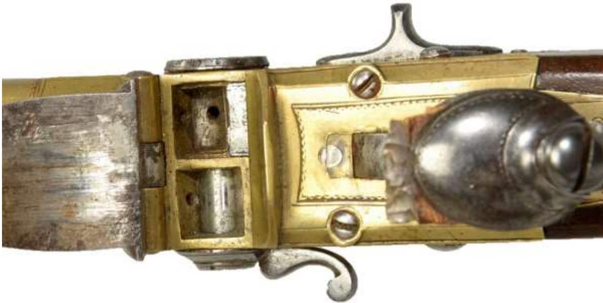
Photos above and below. Perry 4-barrel tap action pistol from above showing the pans and touchholes with the tap and sliding actions in different configuration to fire different barrels. Note the rotating tap action lever on the left side of the frame and the sliding lever on the right side.
