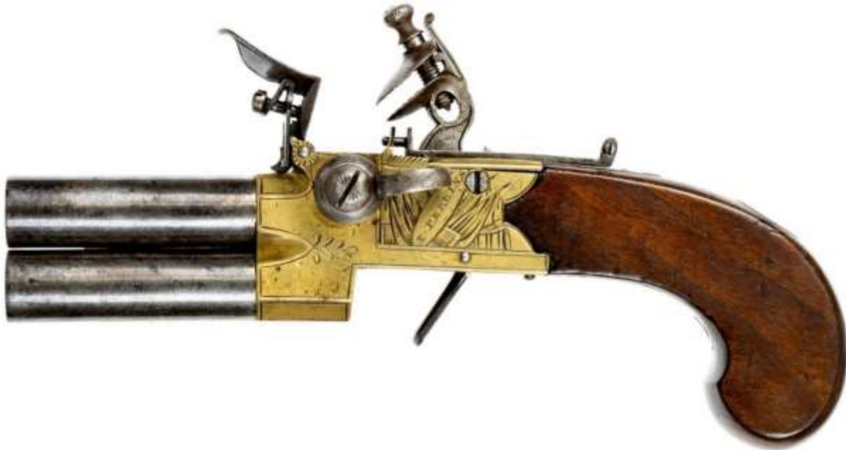
Above and Below - Tap action pistol by Thomas Perrins of Windsor, England. Brass frame, about .44 caliber, made after 1813. This is typical of a late model tap action, two-barrel boxlock pistol with a disappearing trigger, flat sided walnut butt, sliding safety behind the cock and tap action lever on the left side. It is 7 3/8" long with 2 3/16" long barrels. Photos Tim Prince, College Hill Arsenal.
