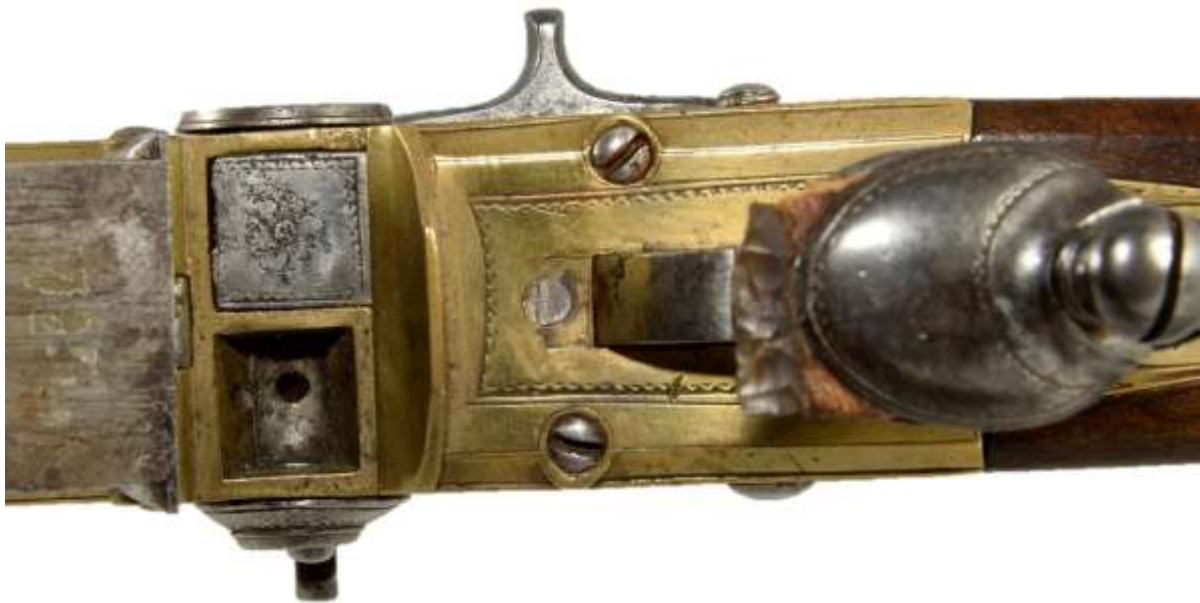
Photos above and below. Perry 4-barrel tap action pistol from above showing the pans and touchholes with the tap and sliding actions in different configuration to fire different barrels. Note the rotating tap action lever on the left side of the frame and the sliding lever on the right side.
