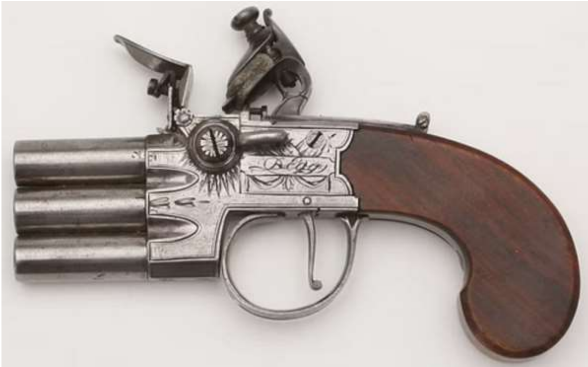
Three-barrel tap action pistol by Durs Egg. Note that the three barrels are arranged vertically, one above the other. Photo - Private collection.
