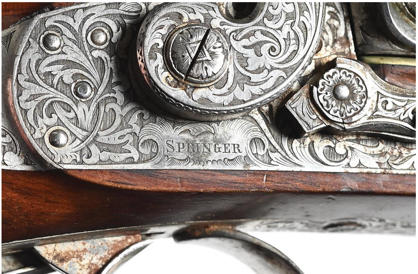
Fig. 9. Right side lock plate. Note name SPRINGER , details of shadowed foliate engraving and hammer block safety. Photo courtesy of Morphy Auctions.
