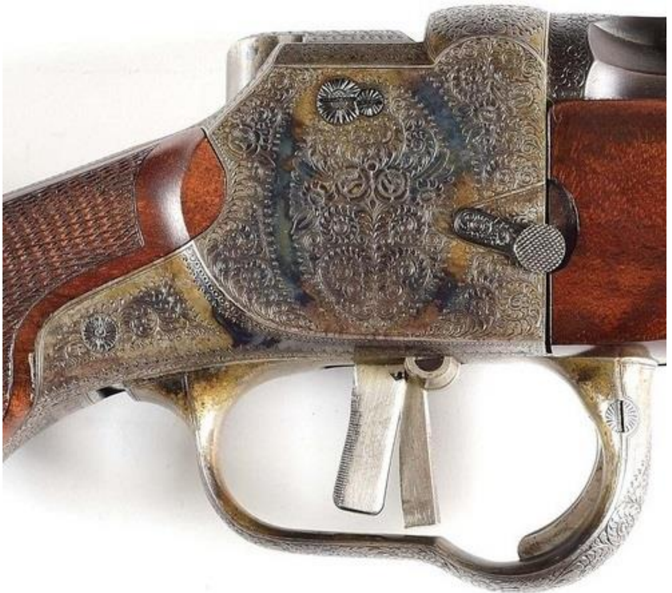
Fig. 35. Enlargement of the color case hardened action, intricate engraving, safety lever, and Heeren trigger guard / lever and Heeren "triggers." Photo courtesy of Morphy Auctions, Denver, PA.
