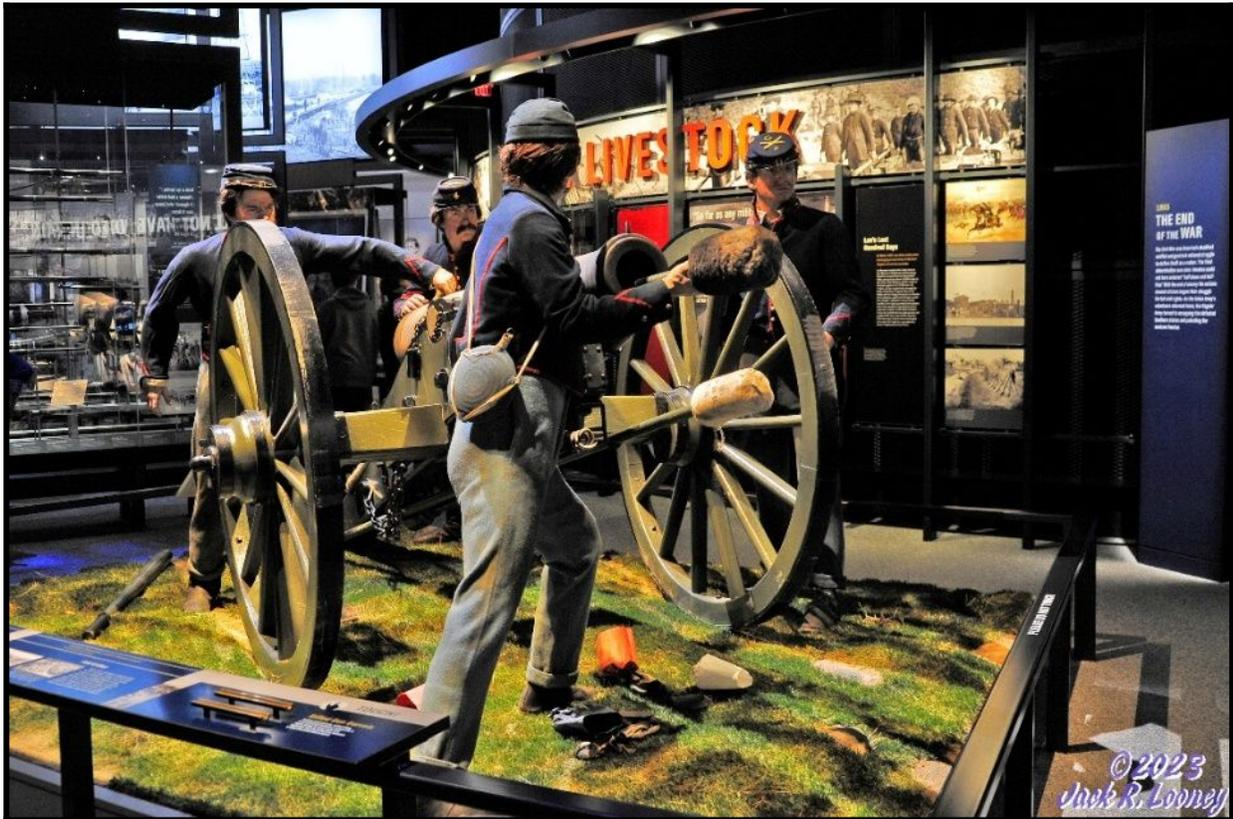
The “Napoleon” was a light and highly mobile smooth-bore muzzle-loading artillery piece of French design (*above right*) adopted by the U.S. Army in 1857. Over 1100 were manufactured for the U.S. Army (most between 1861 and 1863) while another 500 were manufactured for Confederate forces.
