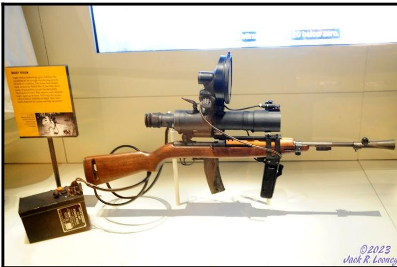
The M3 with M2 sniper scope (*left*) was an early attempt at creating a night vision capability. Deployed right the end of WWII (replacing the first T3 variants), it consisted on an M2 select-fire carbine with an infrared spotlight (on top), television type cathode ray scope to "see" the target, and associated battery pack carried in a backpack. Ungainly and heavy, it had a range of approximately 100-120 yards. The M3 with the M2 sniper scope saw service during the Korean War and into Vietnam.
