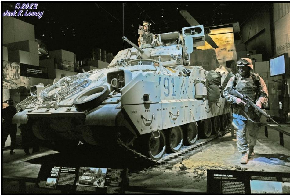
Named for General Omar Bradley, the Bradley Fighting Vehicle (*left*) mounts a 25mm M242 Bushmaster chain gun, two BGM-71 TOW (Tube-launched, Optically tracked, Wire-guided) anti-tank missiles, and an M240 coaxial machinegun. The “upside down V” on the side of the hull was an Allied identification symbol used during Operation Desert Storm in 1991, much like the “Z” seen currently painted on Russian vehicles fighting in Ukraine.
