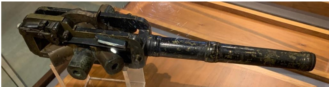
Patent model of the Faries revolving turret “machine gun” from 1829.
