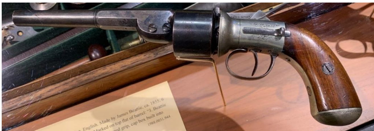
English Thomas Baker percussion revolver with long spur hammer made about 1855.
