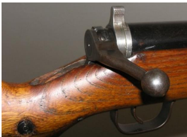
Vz35 bolt in normal position. Rotating safety in front of the bolt handle in the up position. Photo courtesy of Vzduchovka.cz.
