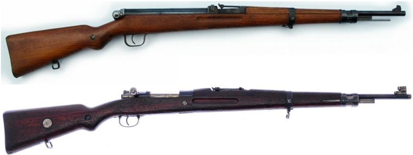
Comparison of Vz35 air training rifle (above) to a Vz24 Mauser rifle made at Brno (below). Top photo Vojensky Historiky Ustav, Praha. Bottom photo courtesy of Joh. Springers Erben.
