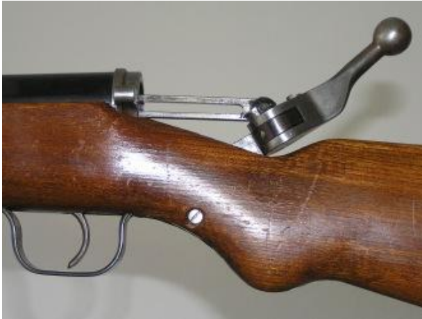
Left - Vz35 bolt in the pulled back and down position to cock the airgun. Photo courtesy of Vzduchovka.cz.
