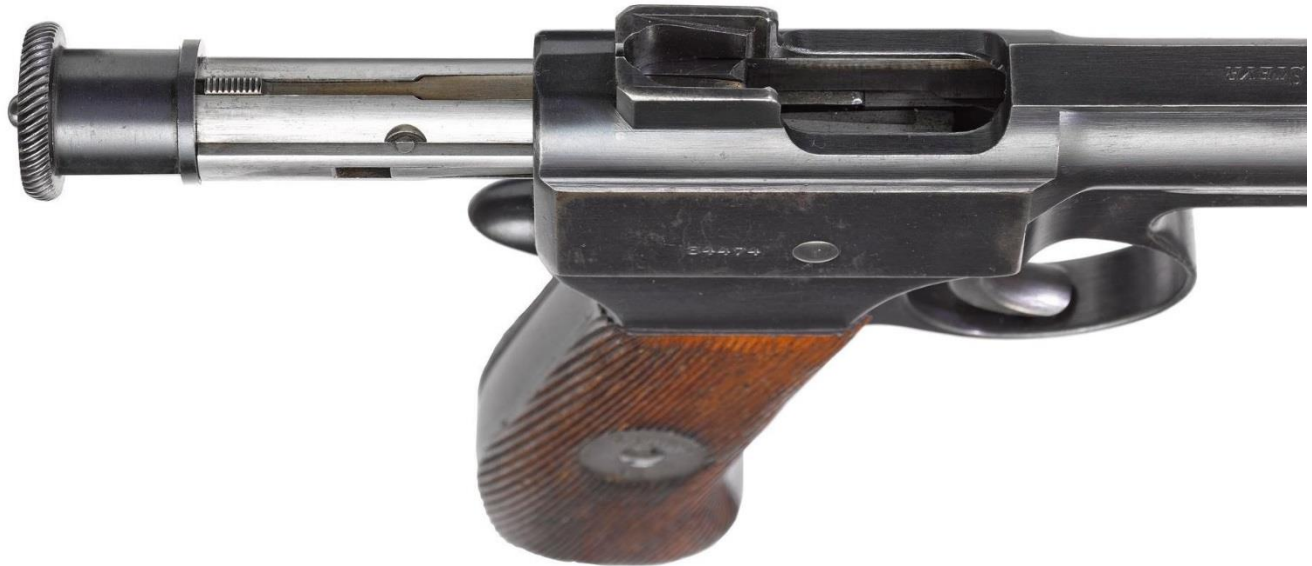
Roth-Krnka (Roth-Steyr) M1907 with bolt open. Photo – Royal Armouries, UK
