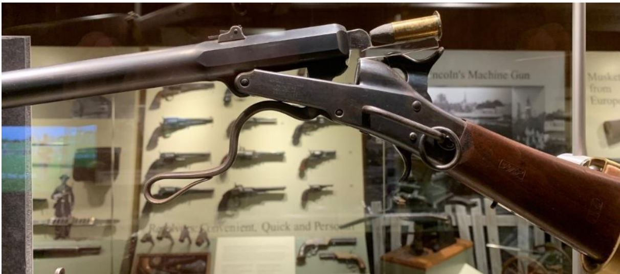
Second Model Maynard carbine with cartridge. The Maynard copper cartridge had a small hole in the rear through which a spark from a percussion cap ignited the powder charge. Invented by Dr. Edward Maynard, a dentist who also invented the Maynard Tape primer, the reliable cartridge could be reloaded about 100 times.
