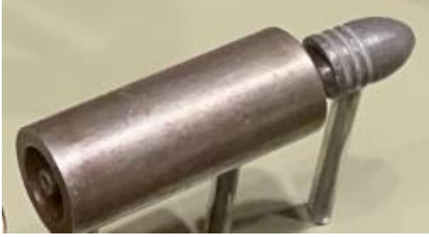
Photo left – Ammunition for the Agar “Coffee Mill” Gun. The powder and bullet were put into a tube with a percussion cap at the rear end.
