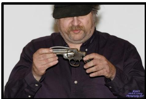
The last revolver presented is an American design - the Maltby & Henley of New York (it is not known whether M&H were the manufacturer or just the retailer). Chambered in .32 Centerfire Short, this DAO has a modular design and disassembles via three screws. An unusual feature is its thumb-wheel safety, which locks the hammer.
