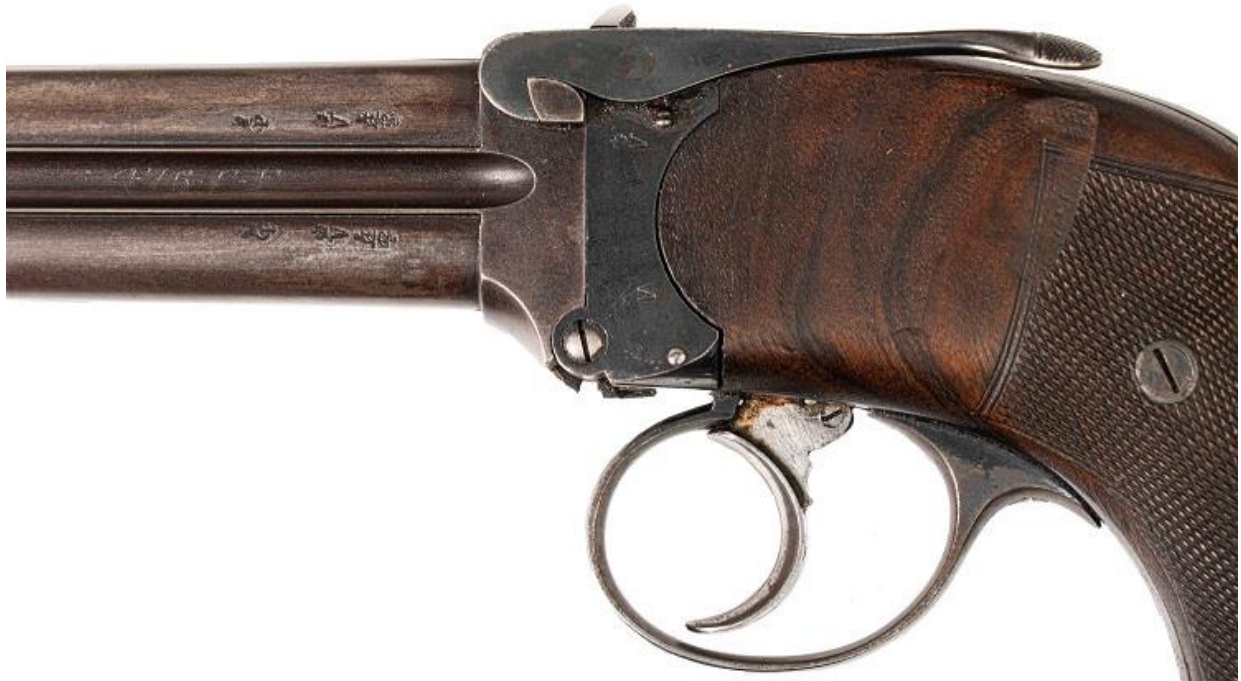
Fig. 4 - Note the lever to open the action, the London proof marks on the barrels and the caliber stamped between the barrels, “.476 CF.” Photo Joh.Springer
