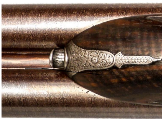
Photo left, detail of engraving on Anson push rod. Note the rose pattern on the banded Damascus barrels.
