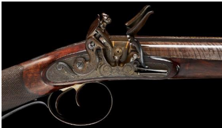
Photo left – Early Purdey flintlock double barreled shotgun number 86. It has rainproof pans (developed by Joseph Manton) and a grip safety. Photo James Purdey and Sons
