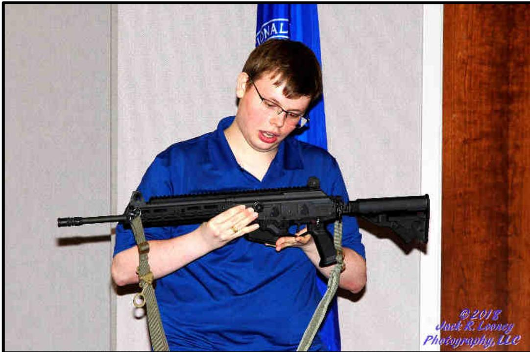
Member 3 also brought in an IWI Galil Ace (*above*). This semi-automatic example was made in Israel on a Micro-Galil receiver and is chambered in 5.56x45 NATO. It has a folding stock, accessory rails, and a last round bolt hold open feature. The Galil, typically chambered in 7.62x39 Russian, has proven popular in replacing AK/AKM-47s in countries with large stocks of that ammunition.
