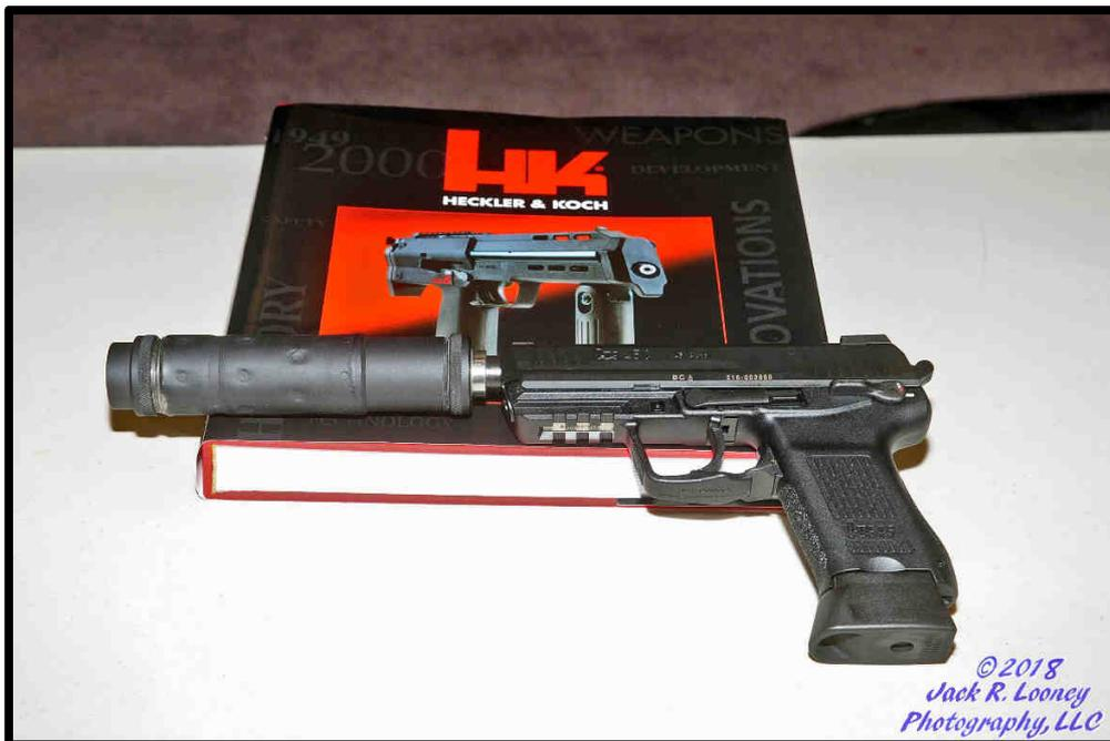
*Also present was this HK Mark 24 Mod 0 pistol with a Knights Armament (KAC) suppressor. Designed as a more compact version of the Mark 23 Mod 0, it utilized an HK USP 45 compact tactical pistol and a smaller suppressor that had a replaceable end cap with wipes (ensuring the smaller can was just as quiet). Made for military trials, the Mark 24 was never adopted/issued. Very few (~100-200) were produced and even fewer are in civilian hands!*
