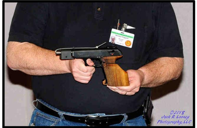
Member 8 shared a unique conversion of an H&K P9S Target Model. This pistol was originally chambered in 9x19 (9mm Parabellum) and was shown as a full kit in the original box. Member 8 had a custom 6.5” barrel made for it in .30 Luger. Why go to all the effort for an interesting but somewhat obscure chambering? His explanation was priceless – “because .30 Luger is a bottlenecked pistol cartridge and bottlenecked pistol cartridges are cool!”
