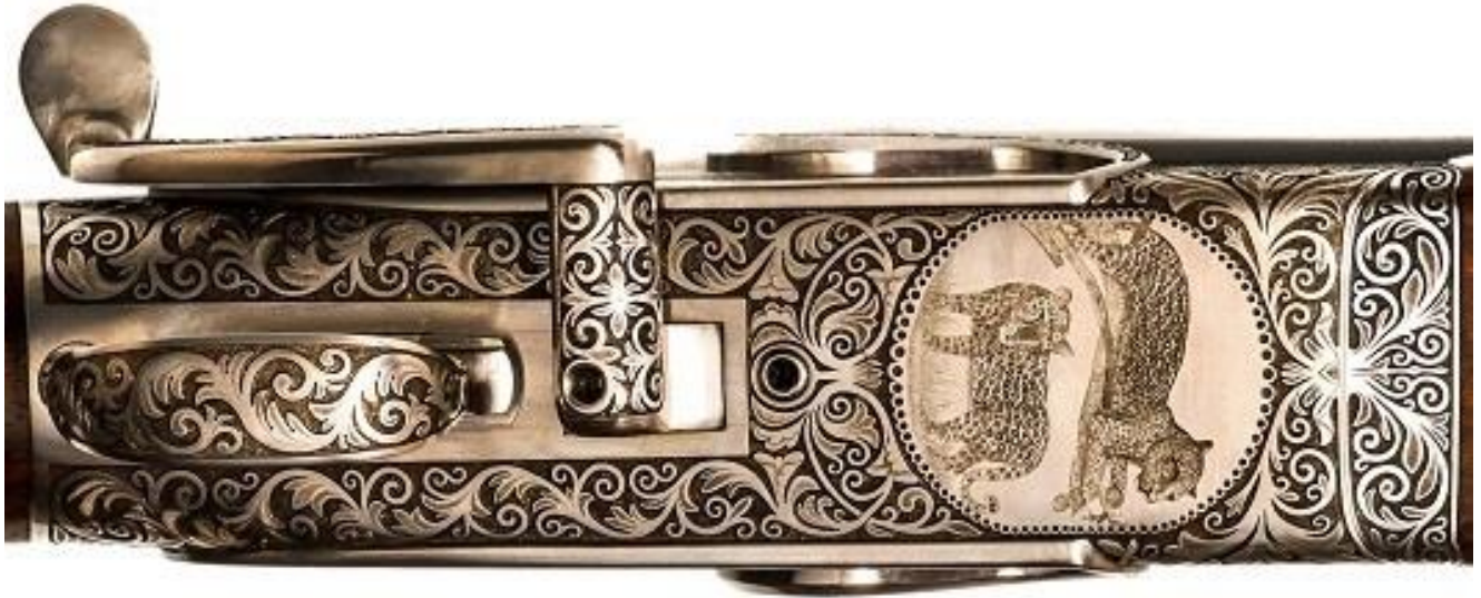
Above and below – bottom of rifle. Note the carved steel cap on the pistol grip, the deep exquisite scroll rocaille carving on the triggerguard, lever and action, and the bulino-style engraving of leopards.
