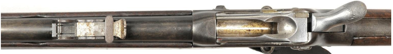
Top view of a Krag-Petersson M1876 action and rear sight. Note that the hammer/lever is slightly offset to the right side of the gun. Photo – kvf.
