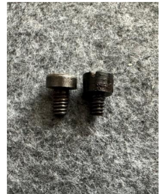
Beretta 1932 grip screw (left), Beretta 1934 grip screw (right)
