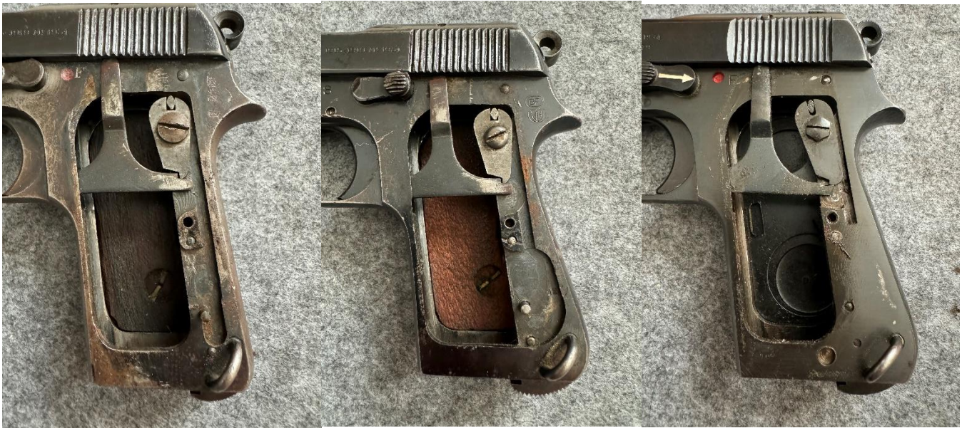
Evolution of the sear bolt, Beretta 1931 large round bolt (left), Beretta 1932 small round bolt (middle), Beretta 1934 hexagonal bolt (right)
