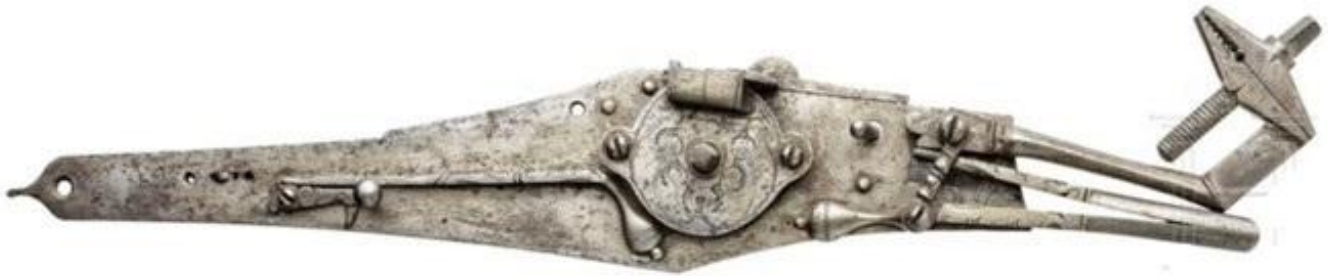
Figure 3. Wall gun wheel-lock mechanism exterior. Lock plate is 37cm long.
