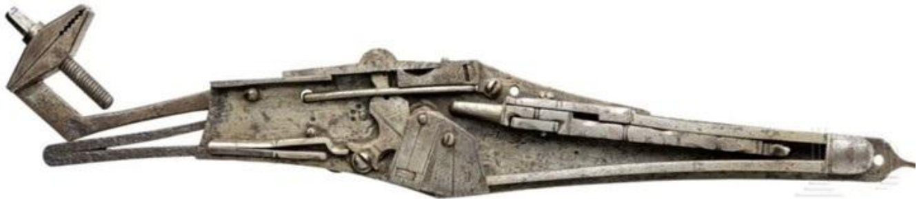
Figure 4. Wall gun wheel-lock mechanism interior
