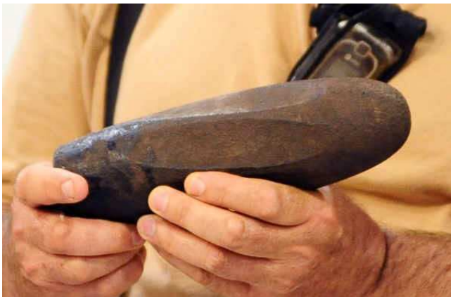
Below: John Morris 2 3/4 inch Whitworth polygonal cannon round made of cast iron.
