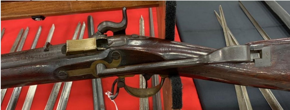
Experimental percussion ignition breechloading alteration of a .54 caliber Mississippi rifle. College Hill Arsenal.
