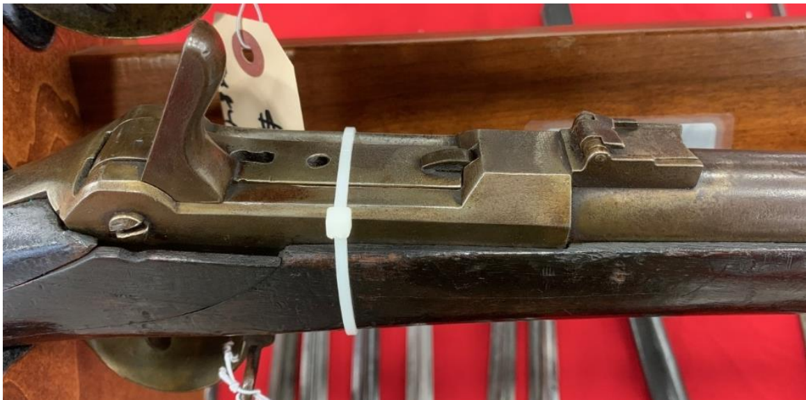
Experimental breechloading .54 caliber rimfire metallic cartridge alteration of a Mississippi Rifle that fired from an open bolt. College Hill Arsenal.
