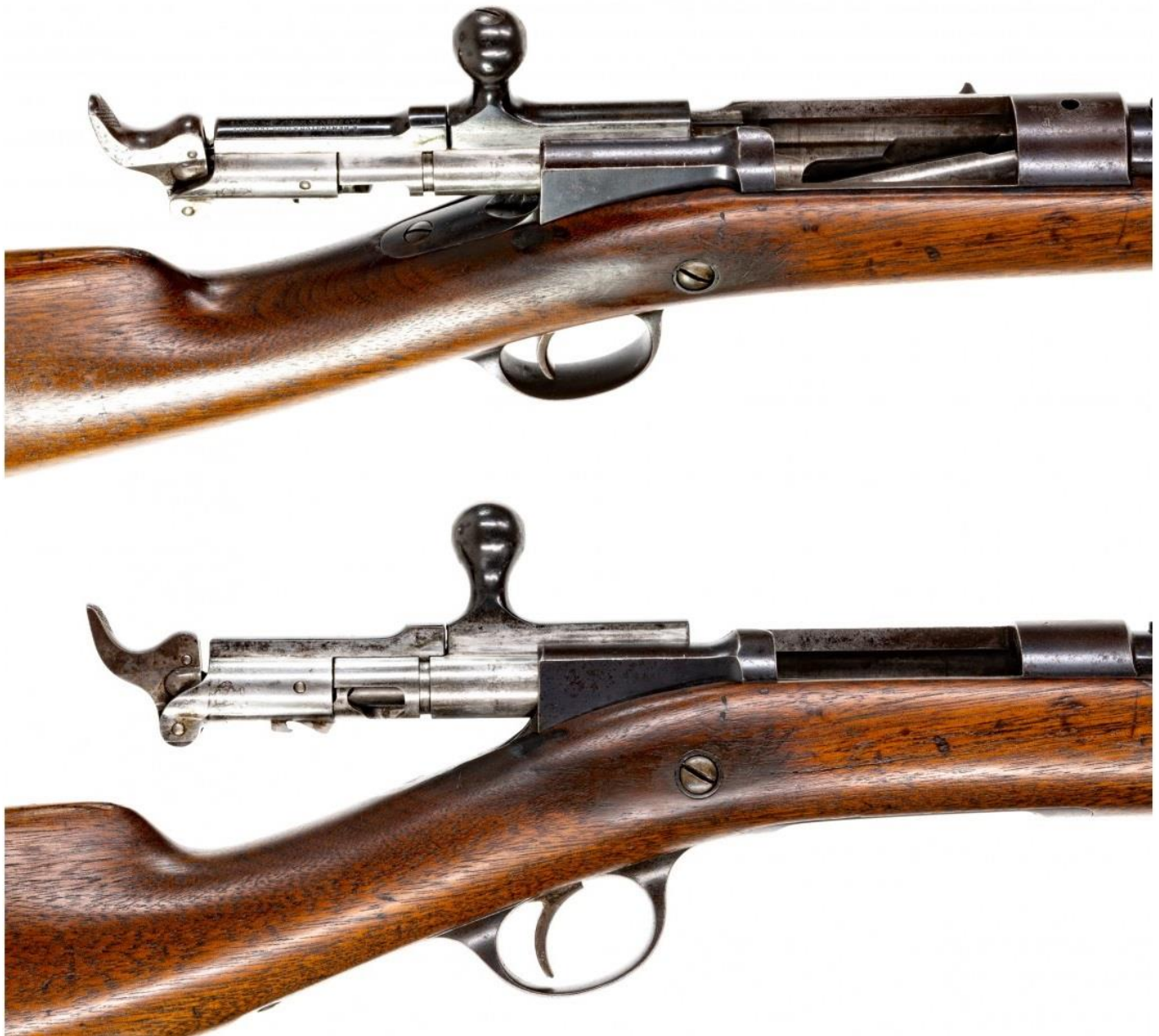
Remington-Keene Indian Police rifle with bolt open. Note the cocking piece on the bolt and, in the top photo, the magazine elevator. The bolt handle is the only locking lug. Photos by Tim Prince.
