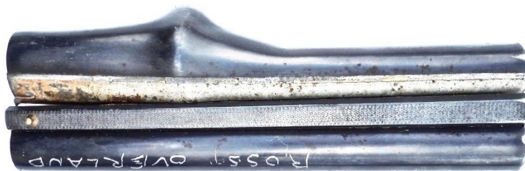
Figure 3. The bulged and split barrel of an Overland (internal hammers), double-barrel shotgun, 12 Gauge, by Rossi, Brazil. The damage was caused by a wad lodged in one of the barrels.
