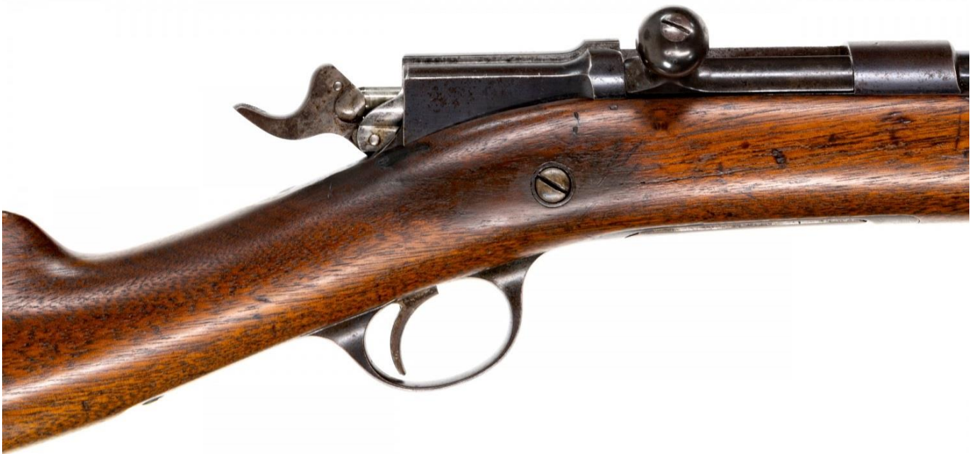
Right side of Remington-Keene Indian Police rifle showing bolt in locked position and cocking piece/hammer cocked. Photo – Tim Prince
