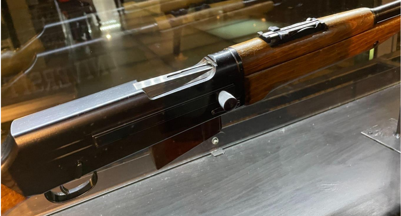
Figure Above: [Notice safety lever right above the trigger guard and the bolt handle adjacent to the receiver]
