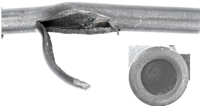
Figure 4. A ripped-open barrel of a Danish Madsen SMG, Model 50, 9 x 19 mm caliber. The damage was initiated by the first bullet lodged inside the barrel - most likely bad ammunition. But, since the case ejected, the gun continued firing additional rounds until it jammed. The first bullet is somewhat visible inside the muzzle.
