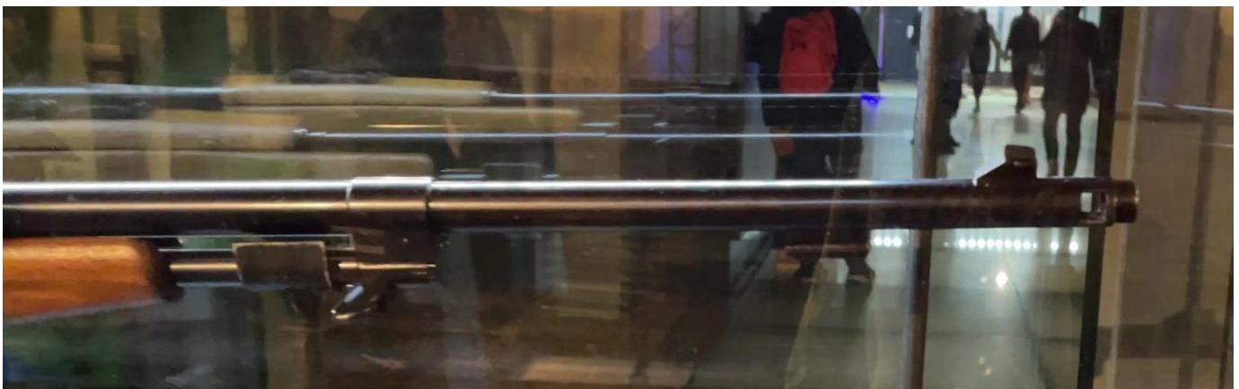
Figure Above: [Notice the gas tube midway up the shaft and the muzzle break at the end of the barrel. The bayonet lug fits a Polish wz.29 rifle bayonet and the front sight is a typical Mauser design]
