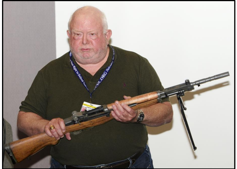
Member 3 also brought a James River Armory Beretta Italian BM-59 battle rifle ( at right ). It is semi-automatic and chambered in 7.62/51 NATO. The receiver is marked 2024 and was acquired in 2024.
