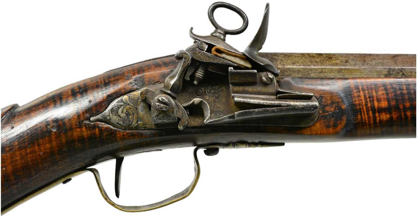
Italian form of miquelet lock of Henri de Tonti's carbine. Photo courtesy of Poulin Antiques and Auctions
