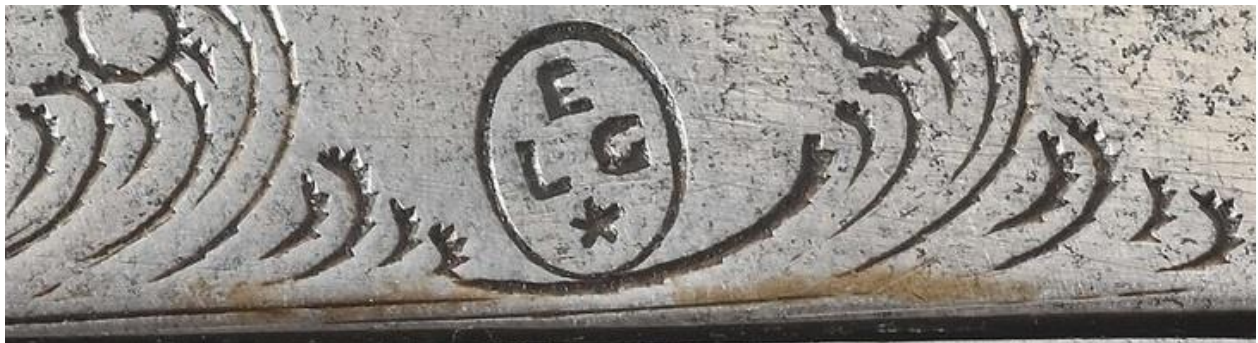
Belgian Liege proof stamp on Chuchu pistol. Photos courtesy of Morphy Auctions, Denver, PA.
