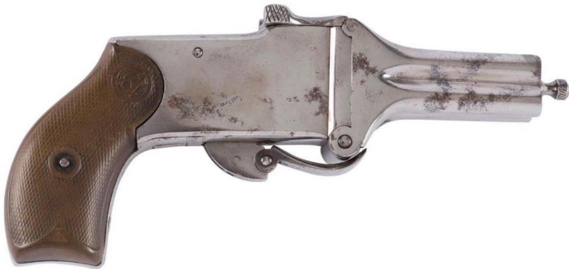
Chuchu pistol with no engraving and trigger folded forward. Photo – private collection.
