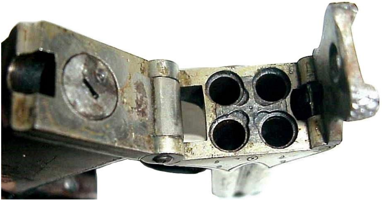
Chuchu pistol with barrels folded down. Note the rotating firing pin on the left and the extractor plate for the manual extractor by the chambers. Photo – private collection.
