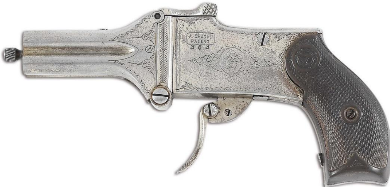
Left side of Chuchu pistol. Note A. CHUCHU /PATENT in a box over serial number 363. Note the knob in front of the muzzles for the manual extractor. Photo courtesy of Morphy Auctions, Denver, PA.
