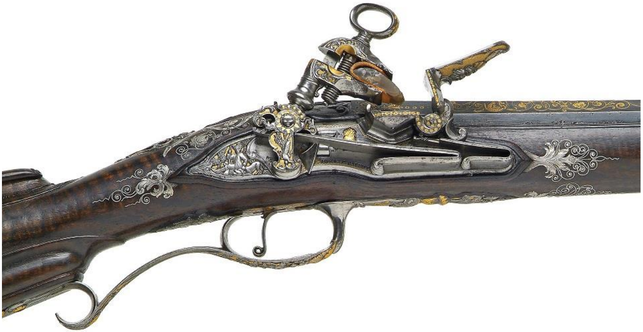
Luxurious Michele Battista rifle made at the state owned Fabbrica Reale di Napoli (Naples Royal factory) in 1775. The exquisite decorations show hunting scenes and the general style of the decoration is Italian-Spanish, due to the Iberian influence that had long been present in southern Italy. Note the Italian style of the miquelet lock. Photo – Grand Curtius Museum
