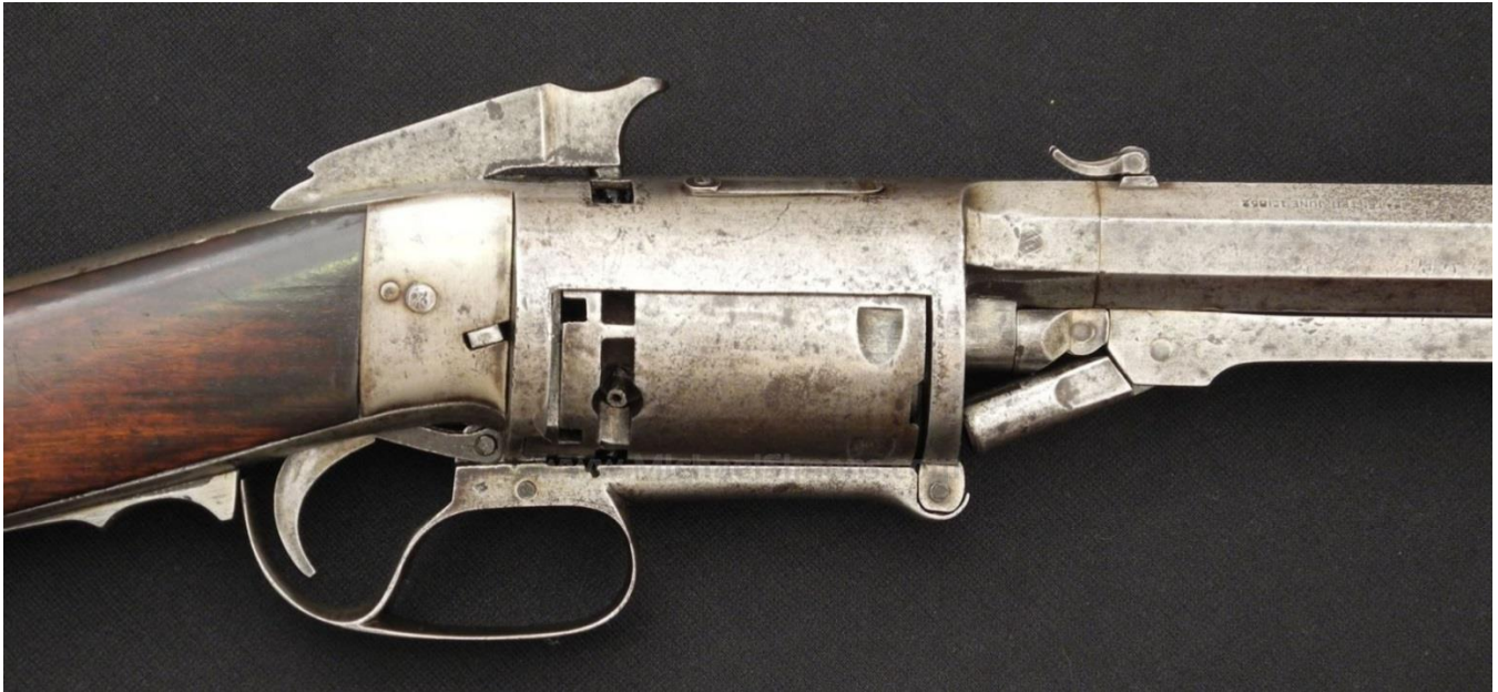
North & Skinner Revolving Rifle with Lever Closed and after firing - Note the wedge raised up behind the cylinder pushing the cylinder forward against the barrel, limiting gas escape. Image from Michael Simens' Historical Antiques.
