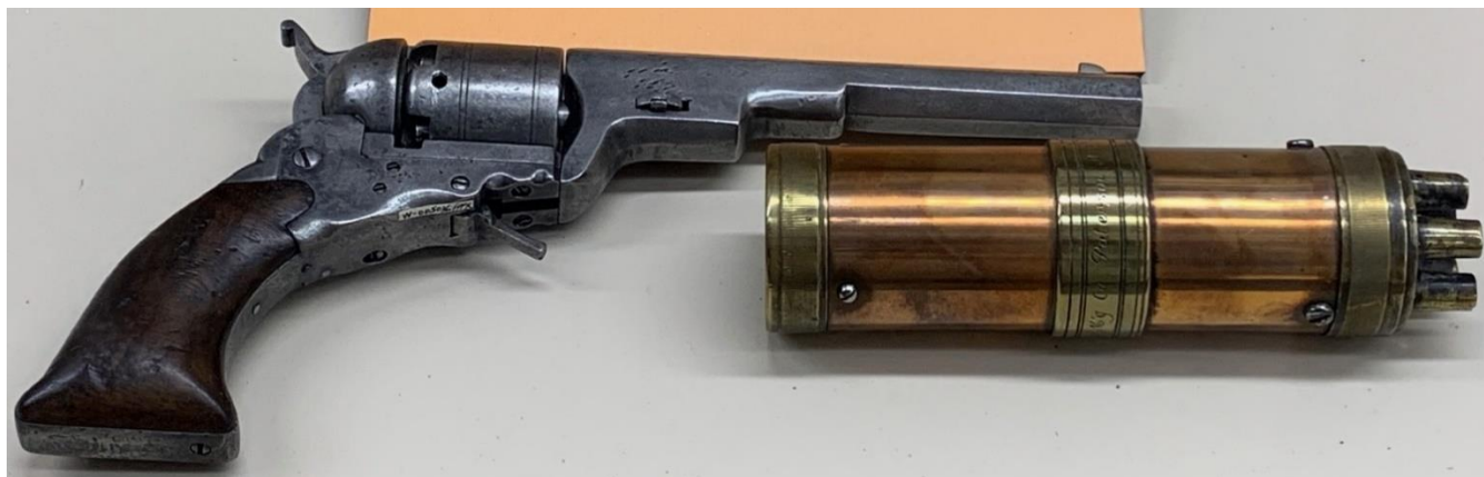
Patterson Colt with charger. The charger allowed simultaneous loading of all five cylinders with pre-measured powder charges. Photo by author.
