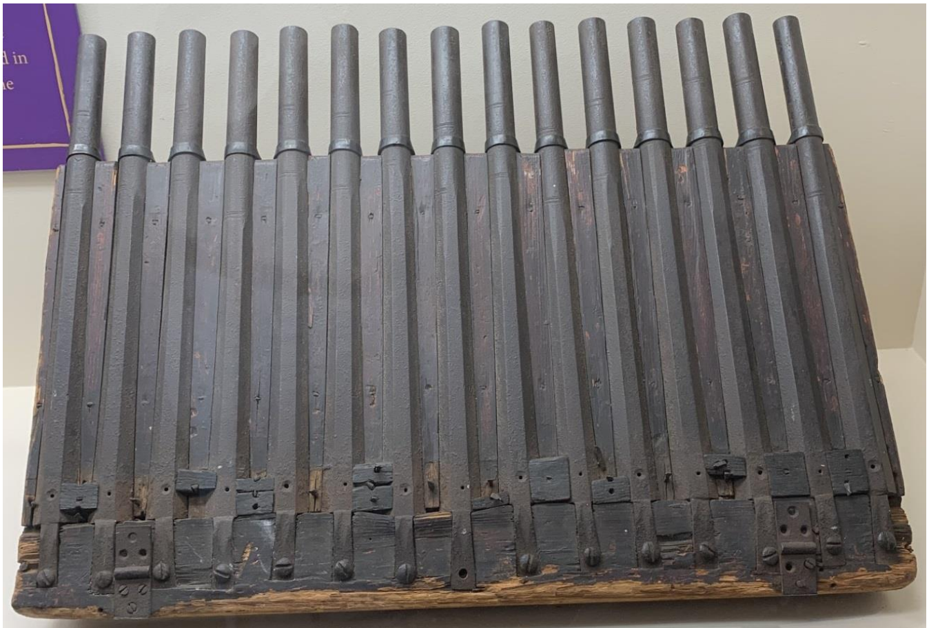
An example of a 15-barrel "leaf" for a volley gun from around 1500. Photo - author.
