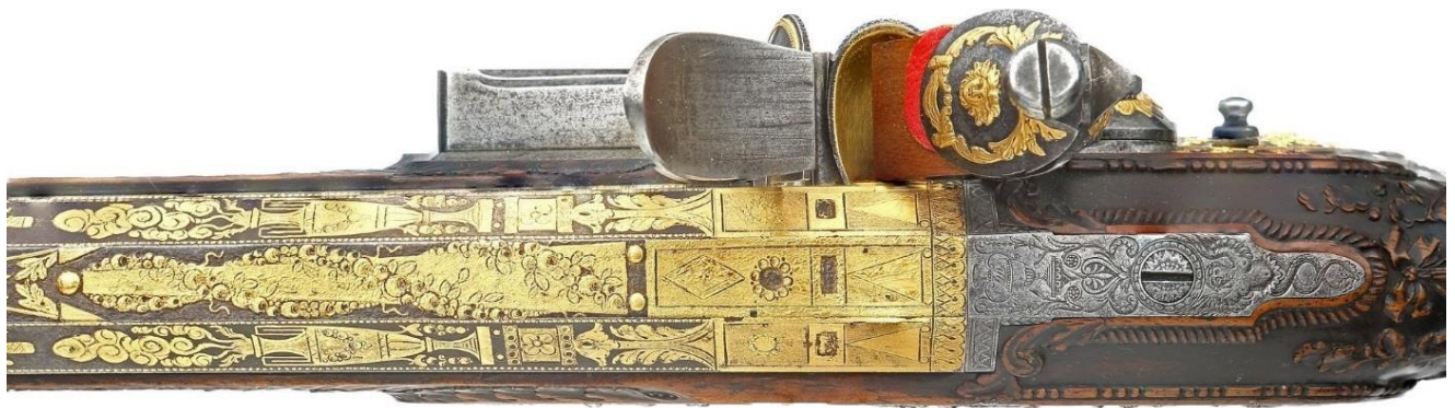
Fig. 13 – Top of gun. Note gold engraving on the cock and gold inlay on the flats of the barrel. The tang is also engraved. Photo Royal Armouries.
