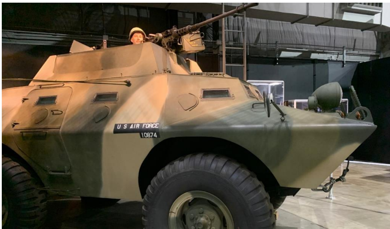
Cadillac Gage V-100 Commando armored car used by USAF Security Police to patrol air base perimeters. Typically armed with one M2 Browning .50 cal. Machine gun, one M-60 7.62mm machine gun and crew's individual weapons.
