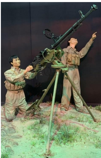
Photo left – Diorama of a DShK-1938-45 heavy machine gun as used by communist forces in a tripod mounted anti-aircraft gun. 12.7mm x 108mm, 600 rounds per minute.
