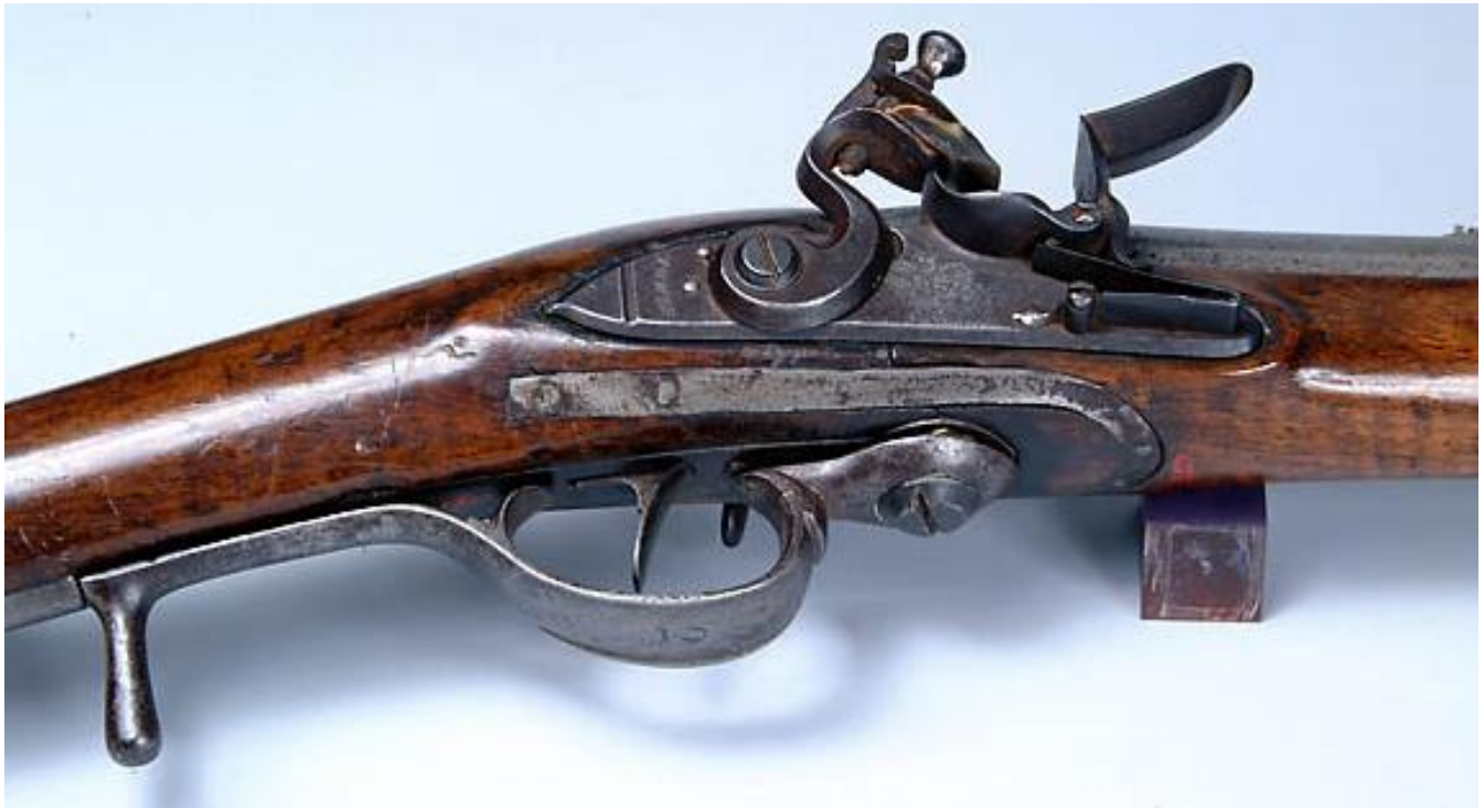
Ferguson Rifle, 1776. British Major Patrick Ferguson patented this breech loading flintlock rifle in England. Only about 200 were made. It has the number '2' stamped on the trigger guard. NPS.
