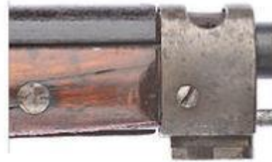
(Fig. 218-2) The stock of the "50 rounds" model m/28 is the most distinctive design variation of the m/28. Fully defined by its double along slots on the bottom of the rifle, it is the only Finnish adaptation of the Mosin-Nagant to adopt this approach to sling fitting.
